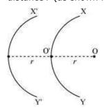
X'Y' can be considered as a virtual reflected ray for the plane mirror. Hence, a point object placed in front of the plane mirror produces a virtual image whose distance from the mirror is equal to the object distance (r).
